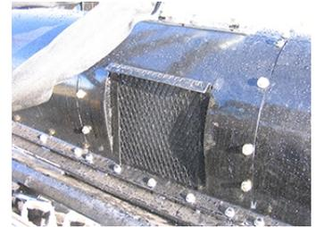
**Hydraulic Cooler**-Equipped with removable debris screen. Located within easy sight of the operator
